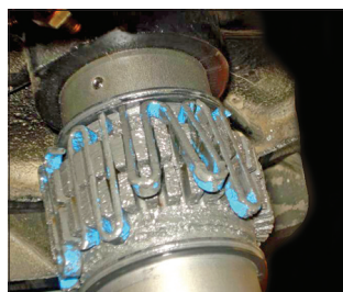
Undersize Coupling for Application
